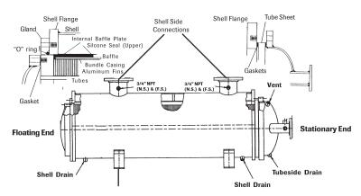
NOTE: Connect a trap to the "cold" side drain for condensing service. Refer to the general arrangement drawing.
