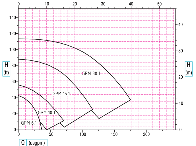
Q (m³/h) GPM. 1 SS316 3500 rpm
